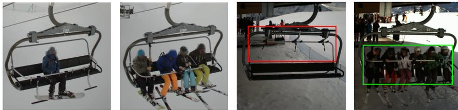
Fig. 5: Example images from our chairlift dataset. The two left images are from chairlift 1 and the two right images are from chairlift 2. The box annotations (open:red and close:green) are provided for the two right images, for illustration.
