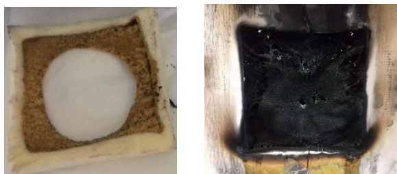
Figure 39: Untreated sample after few seconds in front of a 116 kW burner (left) and sol-gel treated sample after 3 minutes in front of a 116 kW burner (right)
