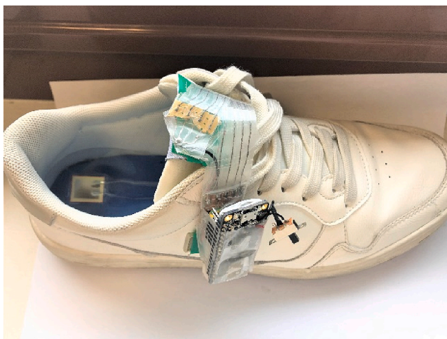
Fig. 21. Prototype of a connected piezoelectric insole integrated into a shoe.
