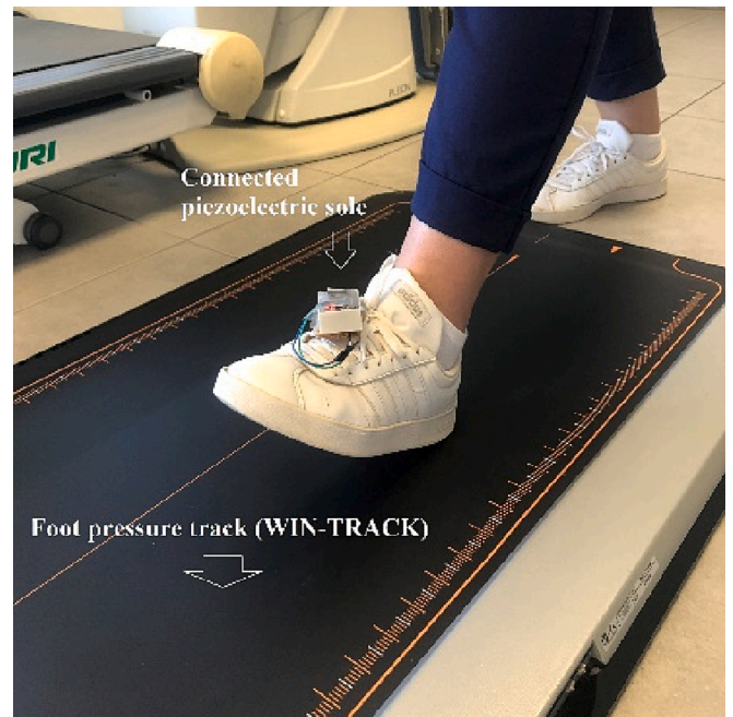
Fig. 26. Walking tests with a connected sole on a podiatric walking mat.
