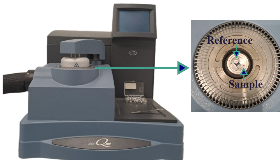
Figure 2.18 – A Differential Scanning Calorimetry Q100 machine used for thermal analysis of materials in the Roberval Laboratory - UTC.
