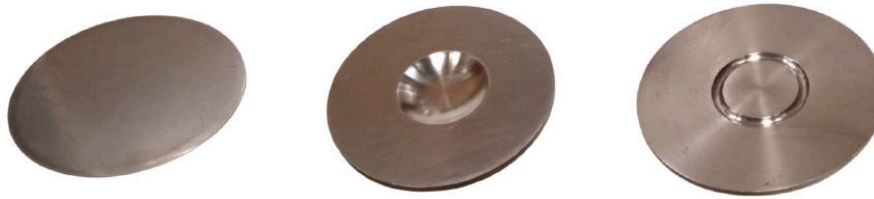
Figure 3.11: Standard, cup and notched disk specimens, respectively.
