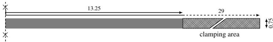
Figure 3.4: Geometry of standard disk specimen (in mm).
