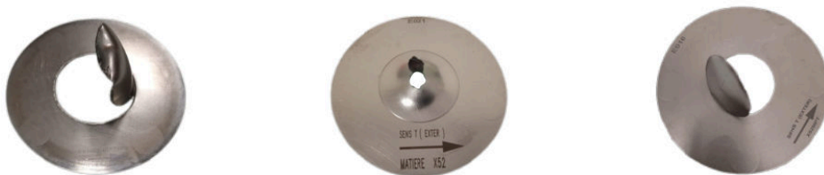
Figure 3.14: Standard, cup and notched disk specimens after failure, respectively.
