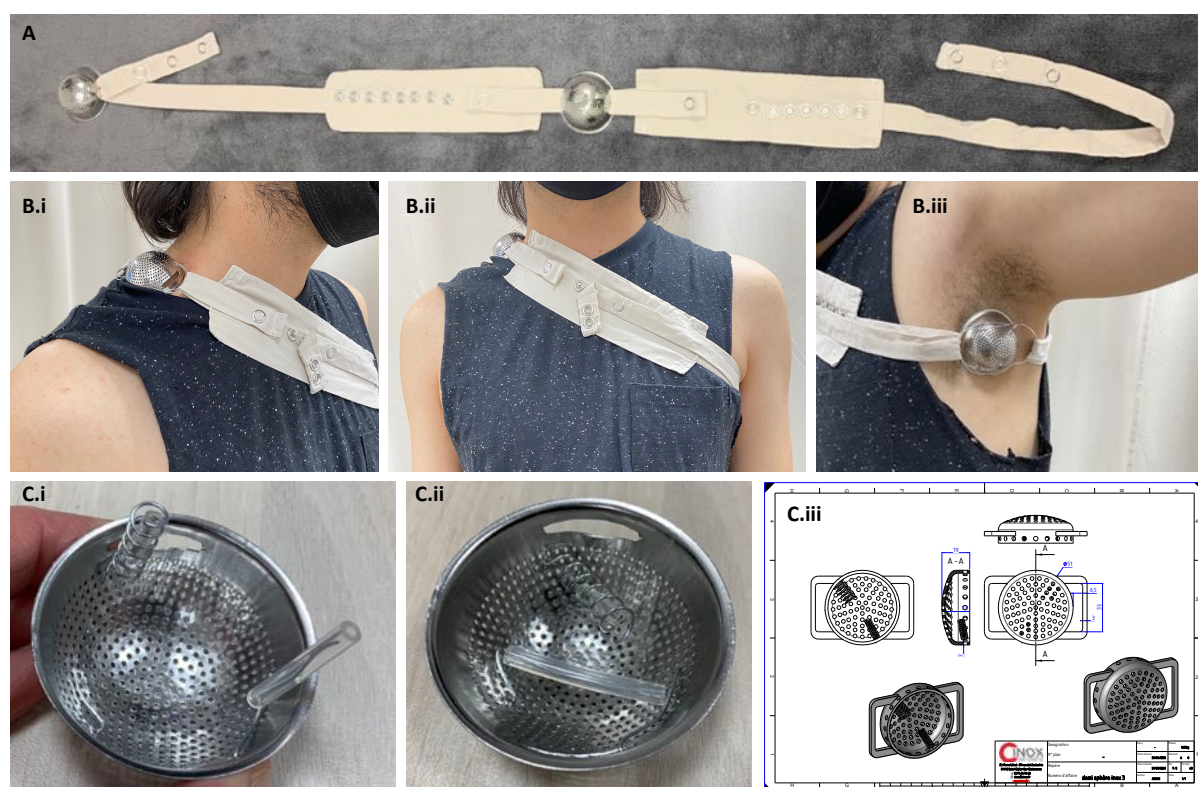
Fig. 10. (A) Our newly developed ABOV device for the collection of VOCs from the human body. (B) Positioning of the device on the axilla and the neck. (C) Detail of the inside of the headspace where springs are used to position the Twisters and Getxent tubes or Powersorbs in suspension in the headspace without touching the skin.
