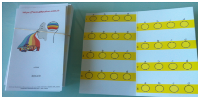
Fig 22. Scratch-and-sniff card used to evaluate the prevalence of ODs in France. Eight odors were used: l -carvone (mint), cis -3-hexen-1-ol (grass), trans -anethole (anise), valeric acid (sweat), alpha -pinene (pine), beta -ionone (flower), isoamyl acetate (banana), tetrahydrothiophene (gas). Odors are trapped in microcapsules and can be released by simply rubbing the printed microcapsule reserve.
