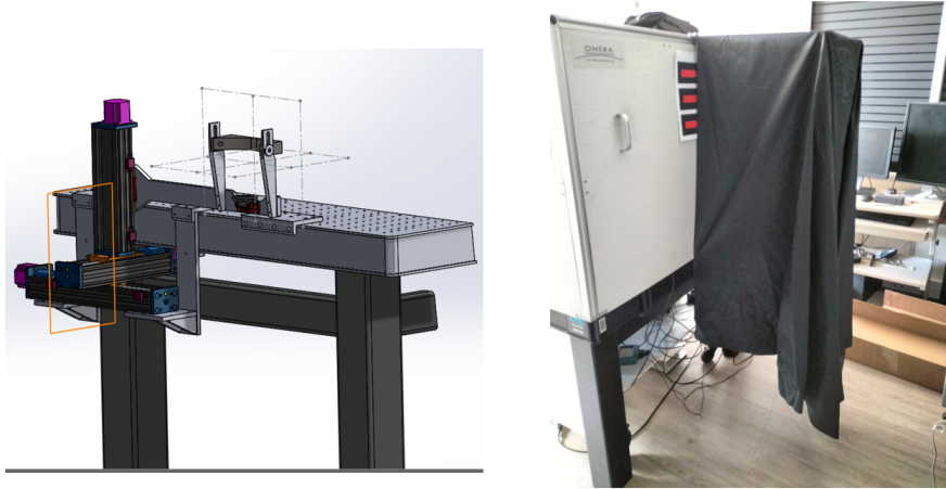
Figure 2.3: On the left, a representation of the new chinrest with 3 motorized axis installed on the system. On the right, a picture of the light-blocking installed on the system.
