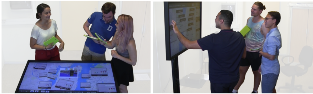
Figure 3.6.: Experimental set-up for the trip planning activity study described in Tong et al. [2017b] : a large interactive surface used alongside tablets. Left: the horizontal condition. Right: the vertical condition.
