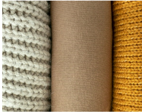
Figure 2.1 – While we are mostly used to think of fabric made of big yarn when knitted garment are mentioned (left and right). For some knitted cloth, the knits, and yarn are practically invisible to the naked eye (middle). (Image from Kozachenko (2020))
