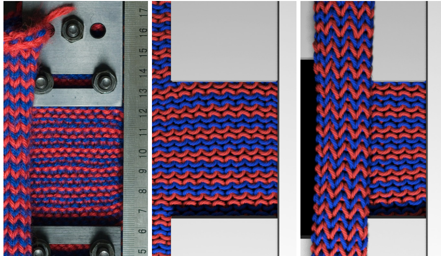
Figure 2.2 – Extension test on fabric knitted with the stockinette pattern. Those tests are performed with different tool: with a real fabric (left); with the cloth model that was used before the introduction of yarn-level models; and with a yarn-level model. Here, the cloth model is not able to reproduce the curling that appears on the left of the real fabric, showing its limitation for the simulation of knitted garment. Images are taken from Kaldor et al. (2008).
