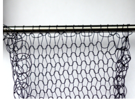
Figure A.2 – Example of an experimental setup where the displacement transverse to the direction of elongation is not constrained. Here, knitted patch is attached to a bar in a way that allow loops to move along the bar. This image was taken from Poincloux (2018).
