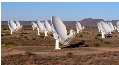
Figure 1.2: (Left) The MeerKAT radio-interferometric array in South Africa. It consists of 64 antennas, and will be a part of the future SKA. (Right) A schematic representation of a radio-interferometric array.
