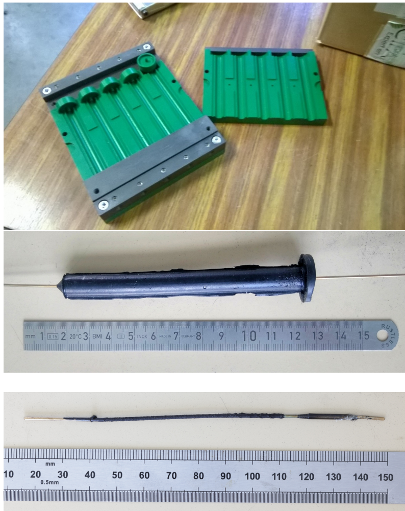
Figure 1.17: Specimens' mold at Michelin (top), a RCAIT sample (middle) and a wire fracture surface after testing (bottom).
