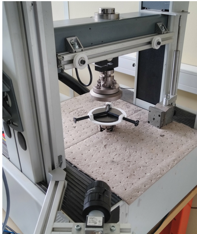
Figure 6.1: Diametrical compression setup for 3 RCAIT samples, with the sample holder in white.
