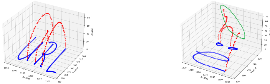
(c) "URL" for ground truth with pen-up movements (d) an "e" for ground truth with pen-up movements, but part of it (in green) is not tracked
