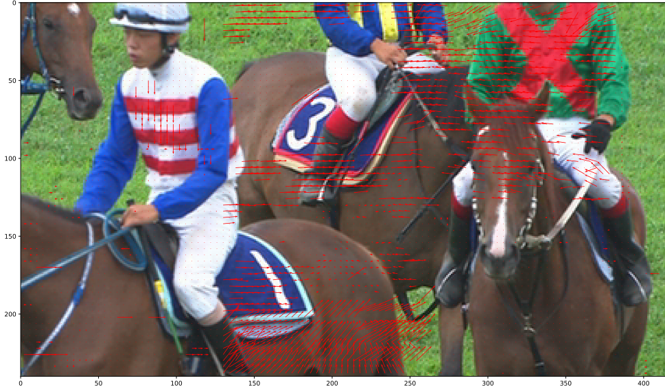
(a) Frame representation combined with its 4 \times 4 MVs directions
