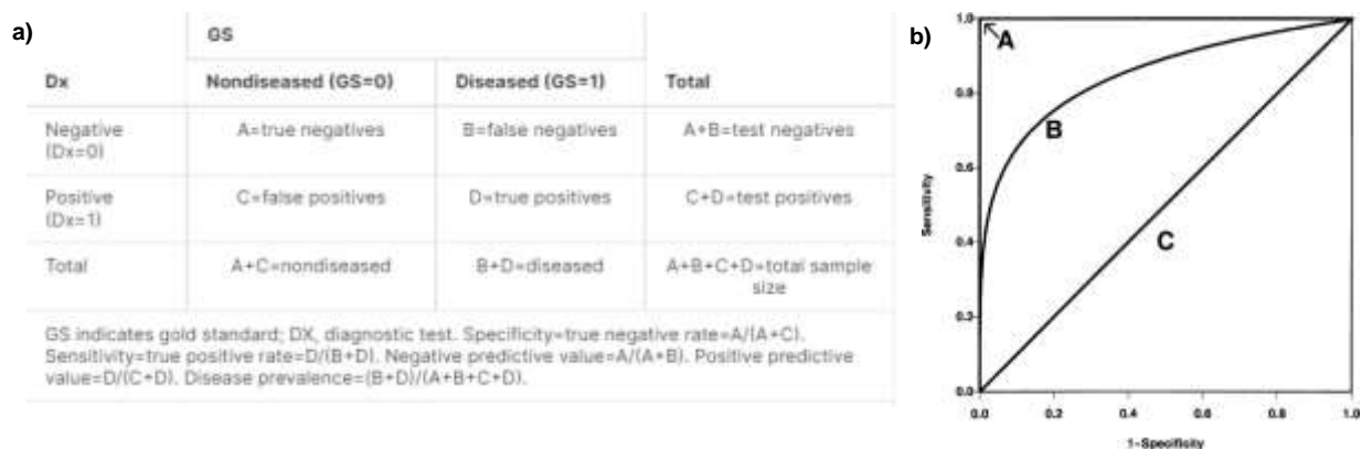
Figure 3.10: a) Decision matrix or confusion matrix generated from the diagnostic test results and the gold standard, to facilitate the plotting of the Receiver Operating Characteristic curve to determine diagnostic accuracy of a given diagnostic test. b) Three hypothetical ROC curves representing the diagnostic accuracy of the gold standard (line A; AUC=1 ) on the upper and left axes in the unit square, a typical ROC curve (curve B; AUC=0.85 ), and a diagonal line corresponding to random chance (line C; AUC=0.5 ). As diagnostic test accuracy improves, the ROC curve moves toward curve A (adapted from Zou, K. H. et al. 211 ).
