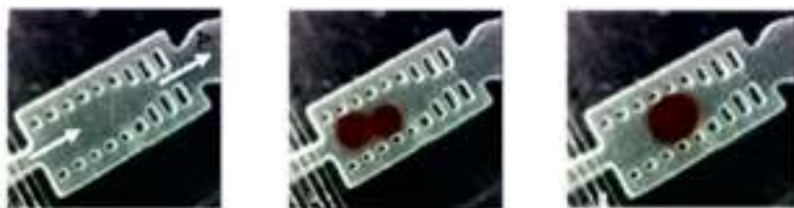
Figure 5.9: Designed microfluidic chip (design 5) that facilitates merging by constriction of two smaller dye solution droplets (100 nL) into a single larger droplet (200 nL), which then moves into the capillary for detection by the camera.
