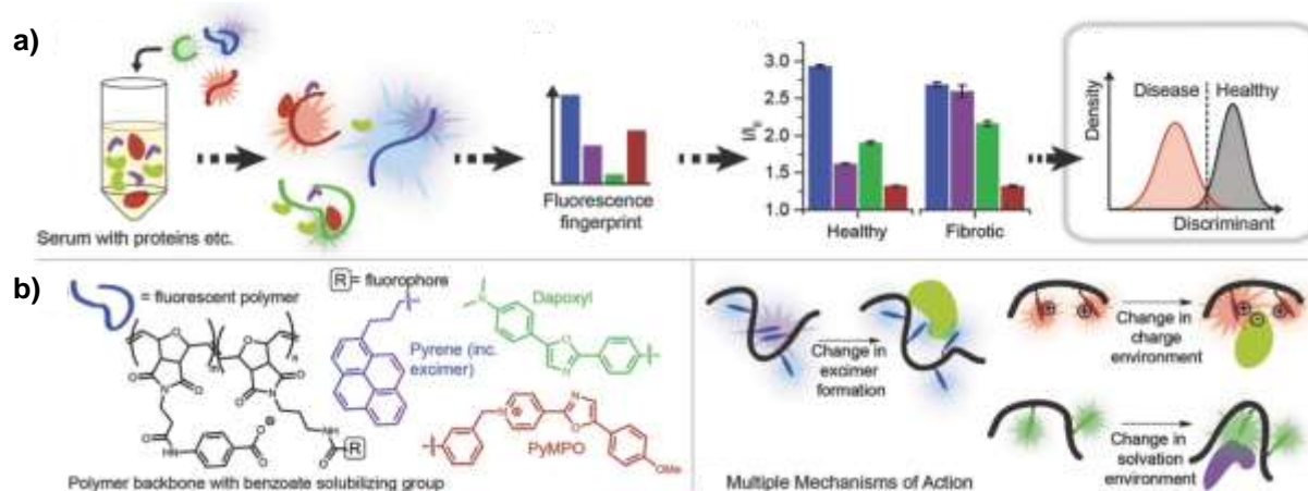
Figure 1.16: a) Schematic illustration of fluorescence fingerprint generation for discriminant analysis for liver fibrosis detection from serum-polymer interaction using an array based sensing approach. b) Polymer structure with three conjugated fluorophores and mechanism of action of the responsive fluorophores generating a four channel sensing array (adapted from Peveler, W. et al. 125 ).
