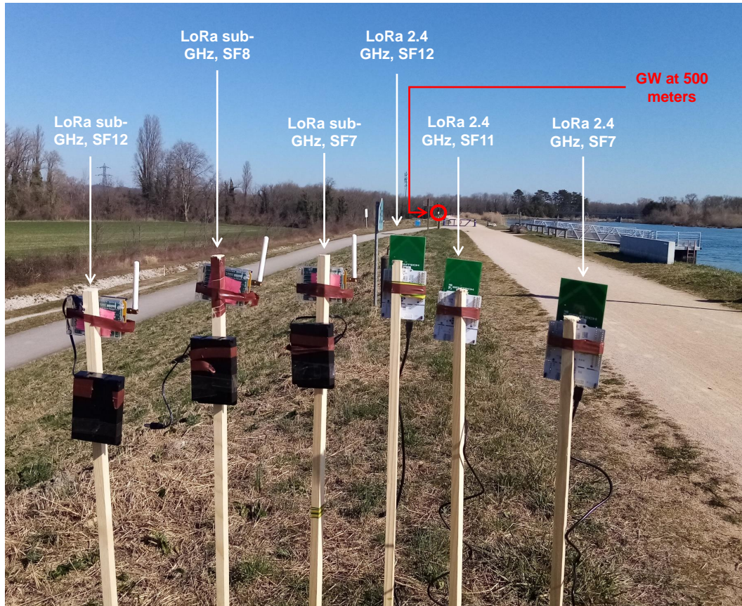
FIGURE 3.10: End-devices placement during communication range experiments.
