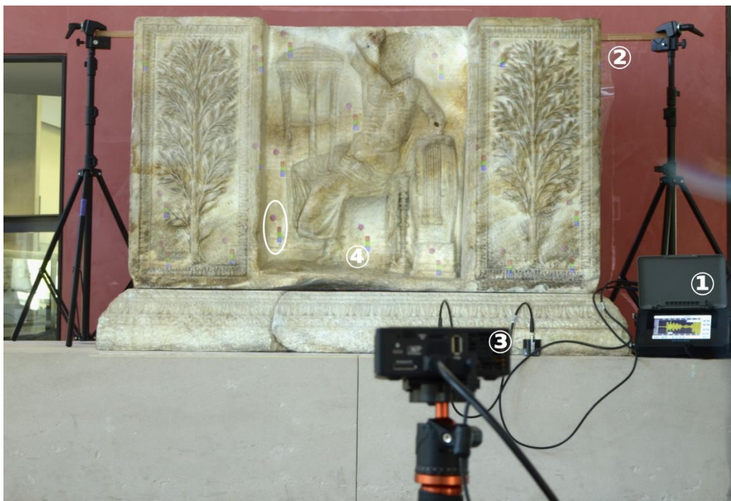
Fig. 61 Experimental set-up for the measurement campaign on the Apollo altar. (1) Time-of-flight measurement apparatus, (2) Melinex® sheet to locate emitter positions at the back of the altar, (3) projector, (4) projected 3D model (gives a blurry aspect to the altar) with each position marked by a combination (circled in white) of a pink circle (point location) and red, blue and green squares (point coordinates).
