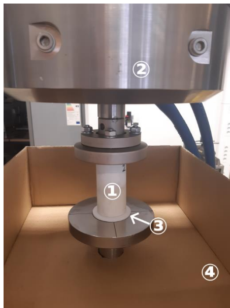
Fig. 31 UCS test set-up. (1) Carrara marble sample, (2) torsional test system, (3) disc of Teflon™, (4) cardboard box to avoid splinters from the sample.
