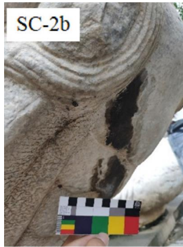
Fig. 4 Black crust. Black crusts on marble sculpture exposed in Beijing Stone Carving Art Museum (Wang et al. 2002).
