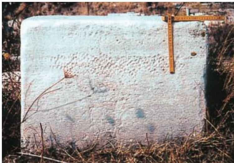
Fig. 5 Salt decay. Small cavities on a marble block in Delos Island, Greece (modified from Chabas and Jeannette 2001)
