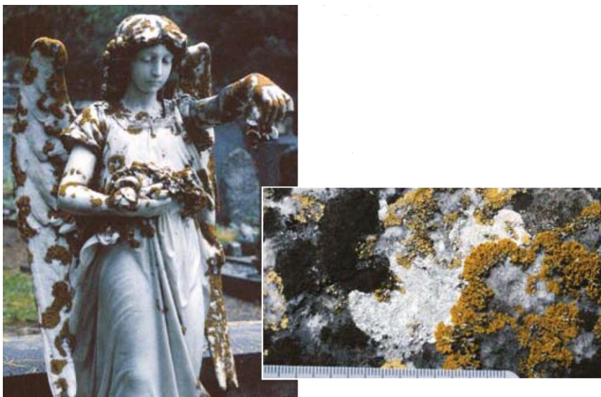
Fig. 3 Biological colonization. Lichen colonization on a marble statue in the Cemetery of Pontresina, Switzerland (ICOMOS Glossary 2008).
