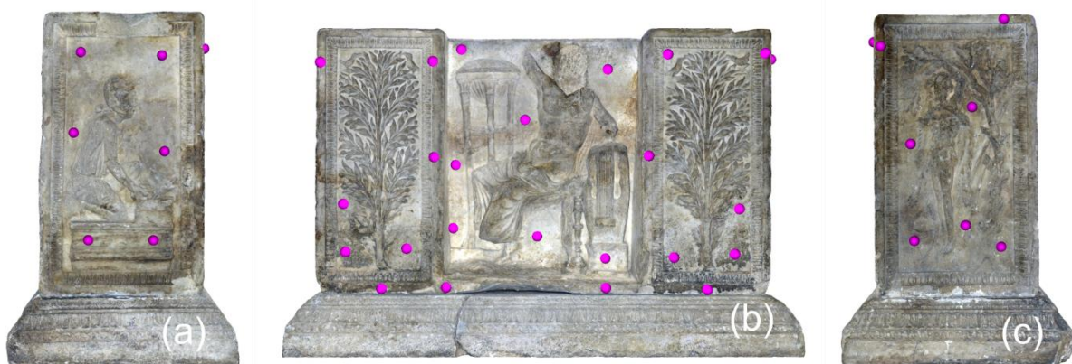
Fig. 63 Receiver positions (pink circles) on the (a) lateral left, (b) front and (c) lateral right sides of the Apollo altar.
