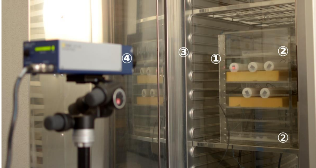
Fig. 2 (Color online) Sample disposition in the experimental set-up. This picture corresponds to the temperature-controlled oven and laser vibrometer part of the scheme of Fig. 1.
