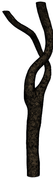
Figure 1.3: The finite element mesh of the vessel used for the simulations.
