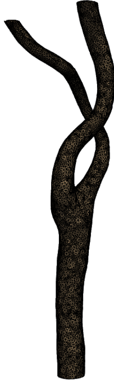
Figure 2.1: The finite element mesh of the vessel used for the simulations.
