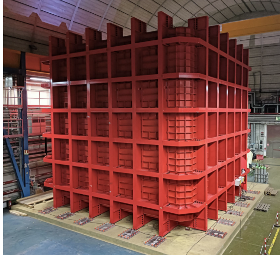
FIGURE 2.5. : Picture of the mechanical structure of the DS20k cryostat completed in 2023.
