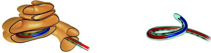
Figure 1.10: A controllable electrode array consisting of a spiral tube (colored in red) and a wire (colored in blue) enclosed within a guiding channel designed for insertion into the scala tympani. [48]
