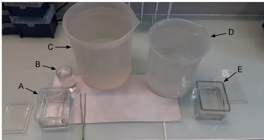
Figure 1. Washing of coated slides. In A we have coated slides in ethanol. B contains ethanol. C and D contain deionized filtered water. E containing deionized filtered water is used to keep rinsed slides before drying.
