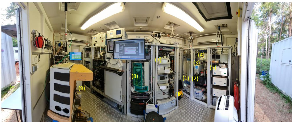
Figure 2.9: PEGASUS (Portable Gas and Aerosol Sampling UnitS) measuring platform: (1) the TEOM (2) Aethalometer (3) water CPC (condensation particle counter), (4) the GRIMM OPC and Nephelometer, (5) CAPS, (6) SP2, (7) HTDMA, (8) PILS (9) ACSM and gas analyzer
