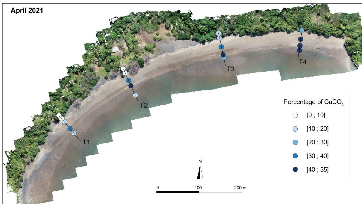
Figure 4. Mapping of transects on Grande Saziley and the location of the surface sand samples associated with calcium carbonate content. Orthophoto by drone.
