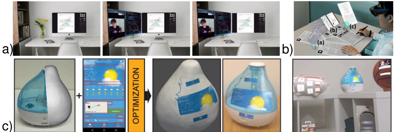
Figure 2.5: Examples of digital information through HMDs are statically a) anchored around a desktop screen [128]; b) placed around physical documents [137]; and c) blended into physical objects [99] a .
