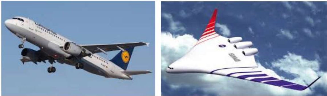
Figure 3.8: Tube and wing (left) and Blended wing body (right) aircraft concepts
