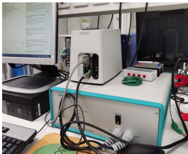
Figure 2.8. Electrochemical workstation (Autolab PGSTAT204, Metrohm) used for electrochemical studies.
