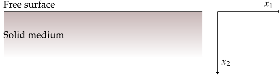
Figure II.2: Diagram showing the coordinate system on a semi-infinite solid structure described by \rho , \lambda and \mu .
