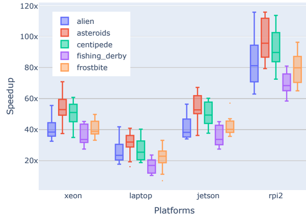
Figure 4.7: Speedup in inference time of the generated code with respect to the library.
