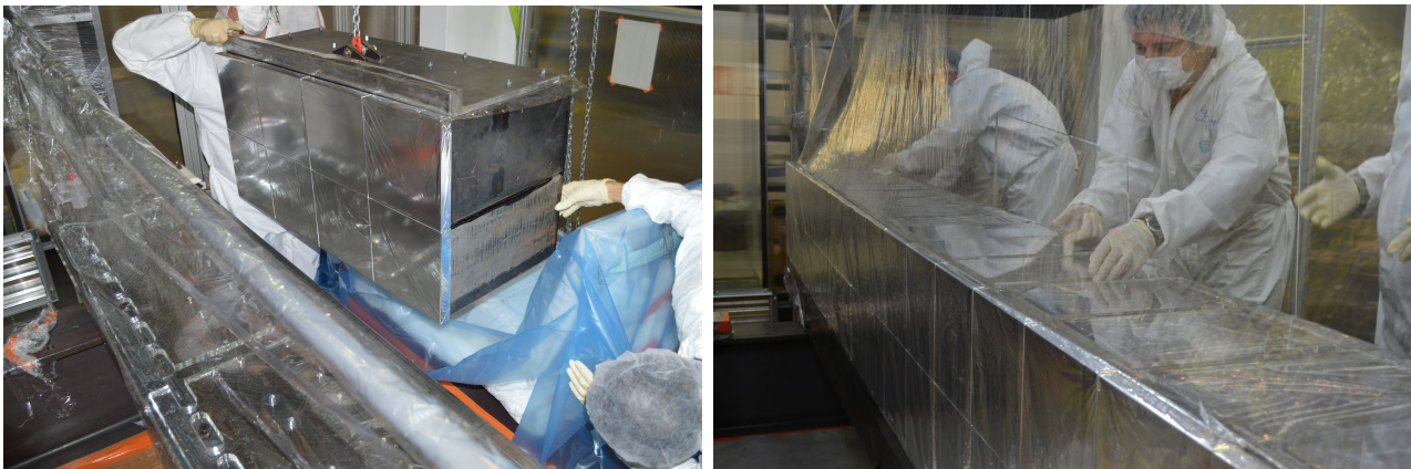
Figure 3.24: (left) Installation of the first calorbrick on the calorimeter frame. (right) Completion of the first row of calorbricks on the first calorimeter frame and installation of the PMMA spacers for the next row.
