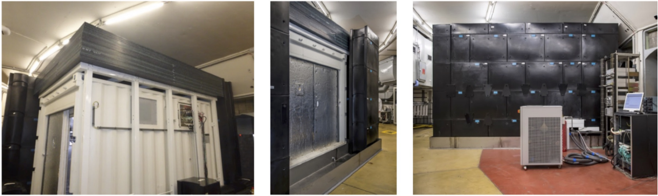
Figure 6.17: Pictures of the detector during its integration at BR2: cooled container (white) and passive shielding (black). The power supplies and DAQ system, together with the chiller used for the container cooling are visible on the side of the detector (front of picture).
