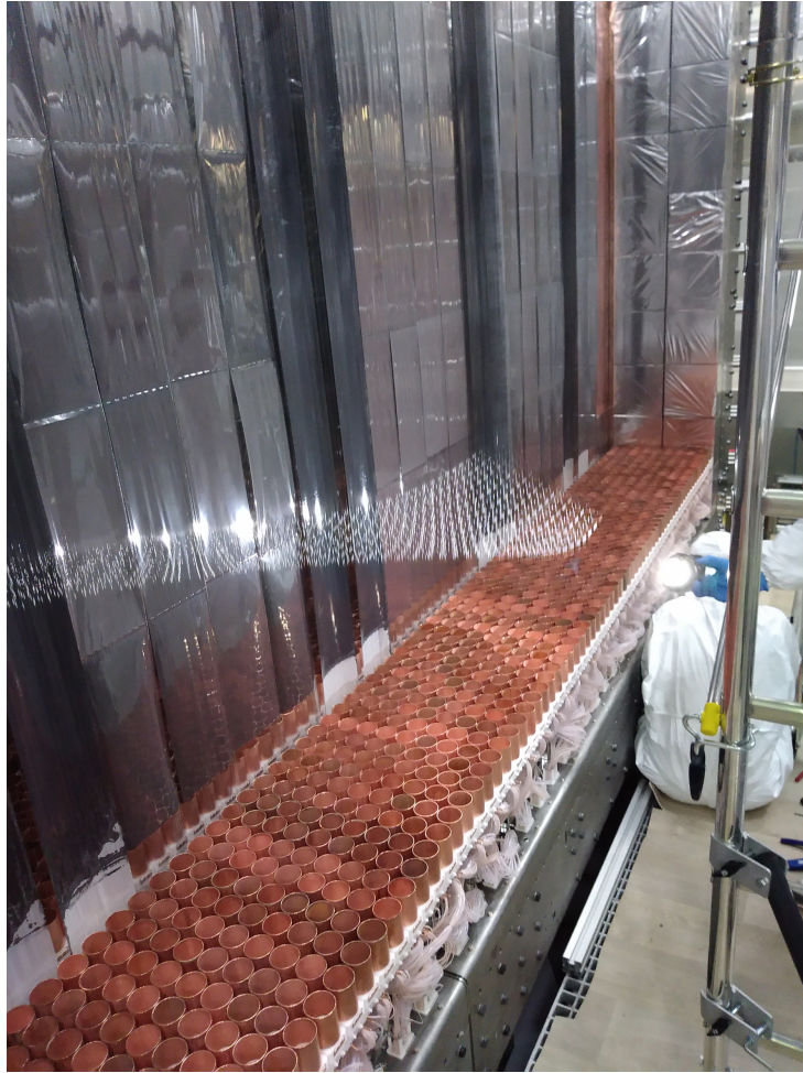
Figure 3.12: Final view of the SuperNEMO tracker closed on the source frame with foils installed, before closure of the main calorimeter wall. A flash light allows to reveal the pattern of the wires in the tracking cells.
