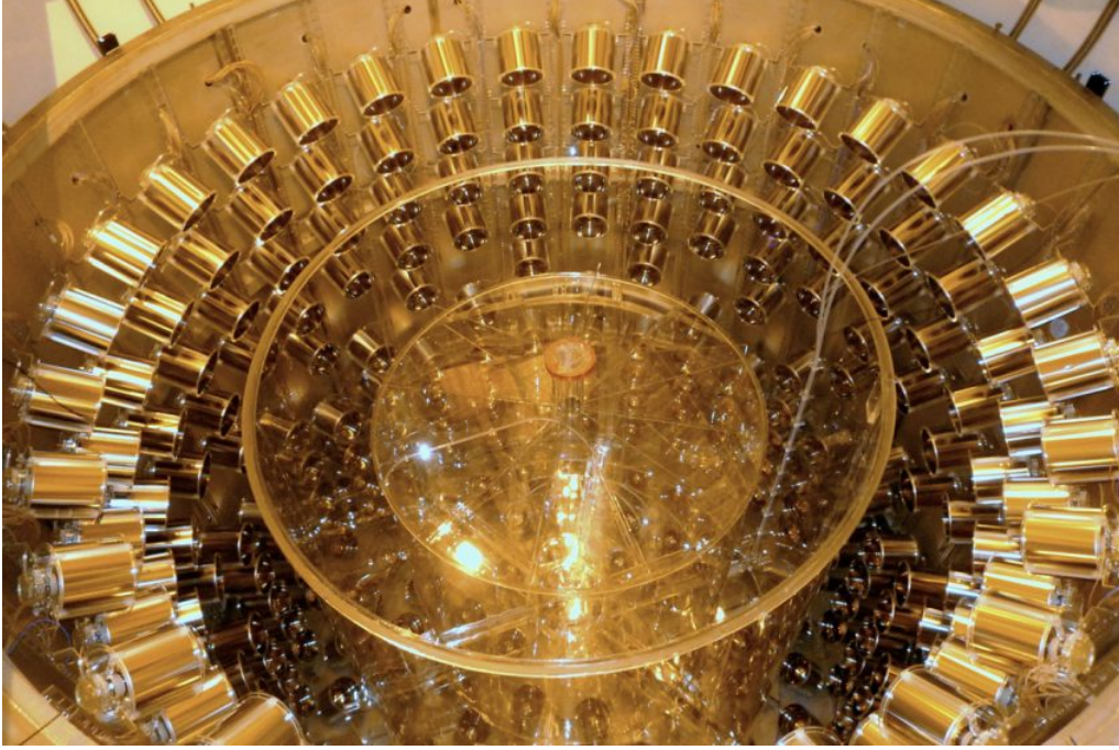
Figure 5.16: Picture of the ID PMTs of the far detector of Double Chooz. The PMTs are encapsulated in cylindrical magnetic shields and acrylic supports. The \nu -Target (GdT) and the \gamma -Catcher (GC) transparent acrylic vessels can also be seen. [Credits CEA-Saclay/IRFU]
