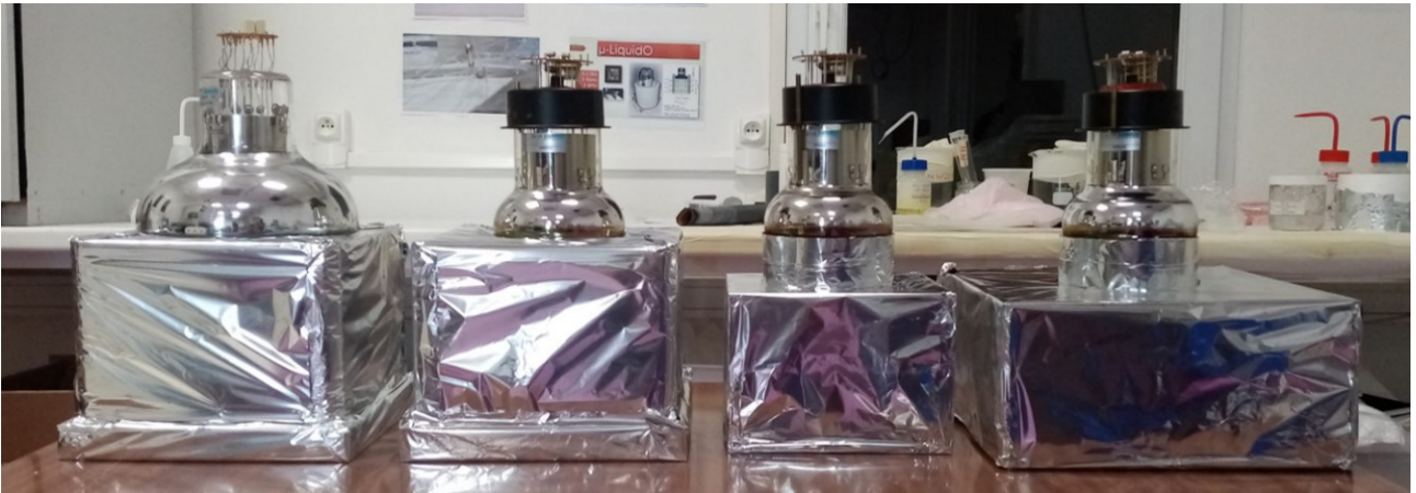
Figure 3.14: Picture of the four types of optical modules used for the SuperNEMO calorimeter during assembly at CENBG. From left to right: M-wall OMs with 8 and 5 inches PMTs, X-wall and G-veto OMs with 5 inches PMTs and PMMA light-guide.
