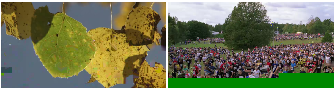
Figure 1.14 Examples of the sequences with the distortion caused by the transmission error
