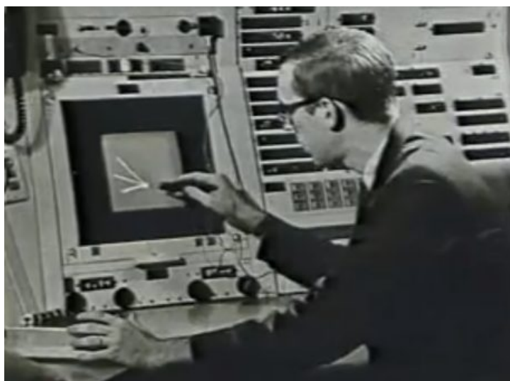
Figure 6: Sketchpad is one of the first CAD applications using a GUI to interact with the users with direct manipulation interactions.
