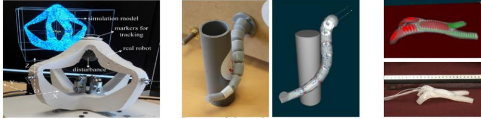
Figure 2.2: Examples of soft robots controlled using FEM: Diamond robot made in silicone and actuated by four cables [Dur13a] (left), a soft tentacle robot actuated by cables [CED17] (middle) and a crawling robot actuated by four pneumatic cavities [GD18] (right).
