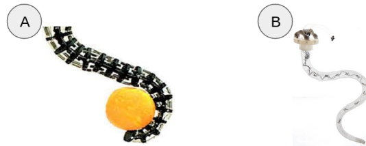
Figure 1.6: Bio-Inspired robots. A) Soft manipulator inspired by the elephant trunk [HW03]. B) Soft manipulator inspired by the octopus tentacle [Las+12].
