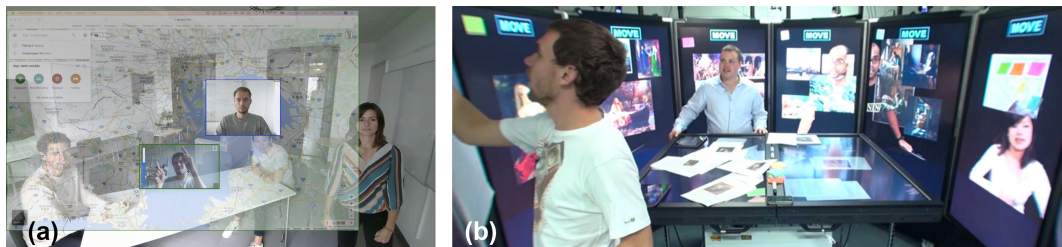
Figure 2.3: Telepresence across large interactive spaces: (a) MirrorBlender blends video feeds and shared screens from remote collaborators (Figure from Grønbaek et al. [Grø+21]), and (b) t-Room uses screens arranged in a circle to overlay remote collaborators' video feeds onto shared digital content (Figure from Luff et al. [Luf+15]).
