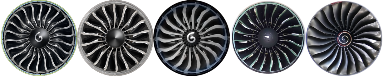
Figure 7.1: Selection of established modern High-Bypass-Ratio Engines (a) GE90 (2003) (22 comp. blades, \varnothing 330cm, BPR 9, 2355rpm, M_r^{tip} 1.2 (nom.)) (b) GEnx (2011) (18 comp. blades, \varnothing 282cm, BPR 9.1, 2560rpm, M_r^{tip} 1.11 (nom.)) (c) CFM LEAP (2015) (18 metallic blades, \varnothing 198cm, BPR 11, 3894rpm, M_r^{tip} 1.19 (max.)) (d) PW1100G (2015) (20 comp. blades, \varnothing 206cm, BPR 12, 3500rpm, M_r^{tip} 1.11(max.)) (e) RR XWB (2013) (22 comp. blades, \varnothing 300cm, BPR 9.6, 2700rpm, M_r^{tip} 1.25 (nom.))
