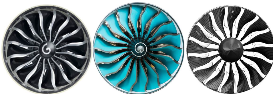
Figure 7.3: Modern industrial low-speed composite fans and Open Test Case ECL5/CATANA (a) GE9x (certified 2020, 16 comp. blades, Ø 340cm). (b) Rolls Royce UltraFan (18 comp. blades / Ø est. 355 cm) (c) ECL5 (16 comp. blades, Ø 50cm)
