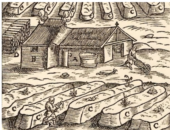
Figure 2.13: German nitrary circa 1580. Leaching deposits (C), where saltpeter crystallizes, are filled with manure and vegetal materials. Source: Wikimedia Commons (2024f)
