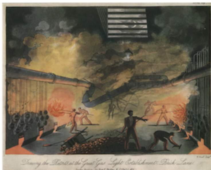
Figure 2.16: Coal gasification, in which ammonia sulfate was extracted from coal. This was performed in gasworks ( "usines à gaz" in French), where town gas ( "gaz de ville" ), also named coal gas, was produced before fossil deposits of methane were exploited. Source: Drawing the retorts at the Great Gas Works at Brick Lane , unknown author, 1821, from Wikimedia Commons (2020)
