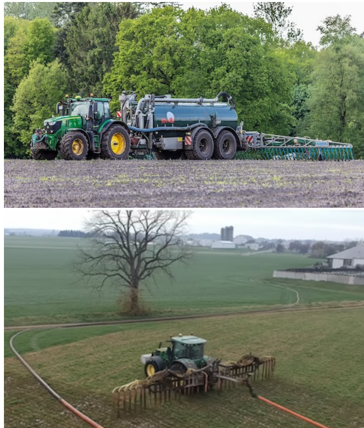
Figure 3.22: Top: slurry spreading with a slurry tanker, whose heavy weight can compact soil and prevent the tractor from entering the field if the soil is too wet. Bottom: slurry spreading from fixed slurry tanker, using a dragline, limiting soil compaction. Sources: Wikimedia Commons (2023c) and youtube (2023)
