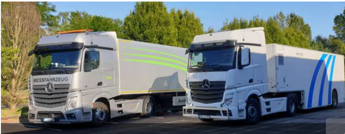
Figure 2.7 – TSDDs, with TSD on the left-hand side & Raptor on the right-one [85].
