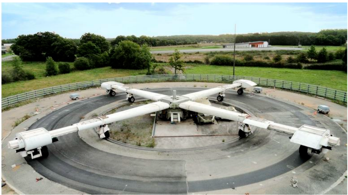
Figure 5.2 – The pavement fatigue Carousel at Univ. Eiffel Nantes [144].
