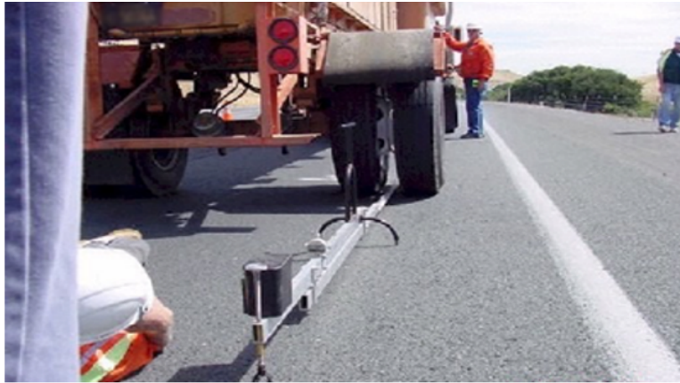
A : Benkelman beam (Static nature)
