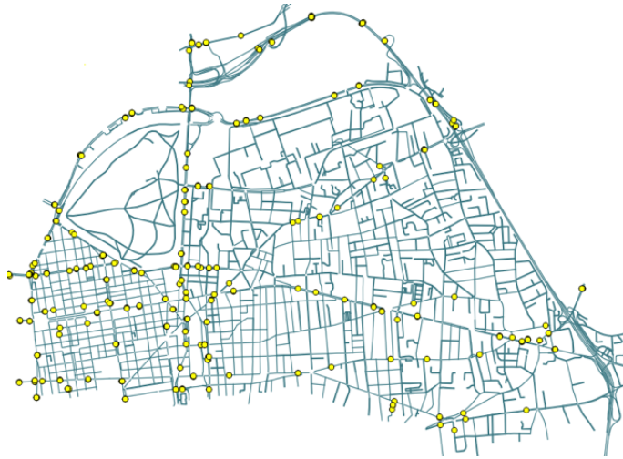
Figure 1.2: Spatial distribution of traffic sensors on the road network of Villeurbanne and two districts (the third and the sixth) of Lyon (figure courtesy of [RCS20]). Yellow dots represent the locations of traffic sensors.
