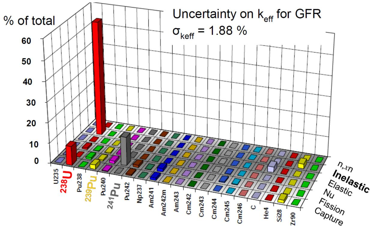
Figure 1: Break down of uncertainty contributions (in %) associated with the total combined uncertainty on the  $k_{\text{eff}}$  of a Gas Fast Reactor (GFR) by isotope and reaction channel. (From reference<sup>Page 5, 5</sup>.)
