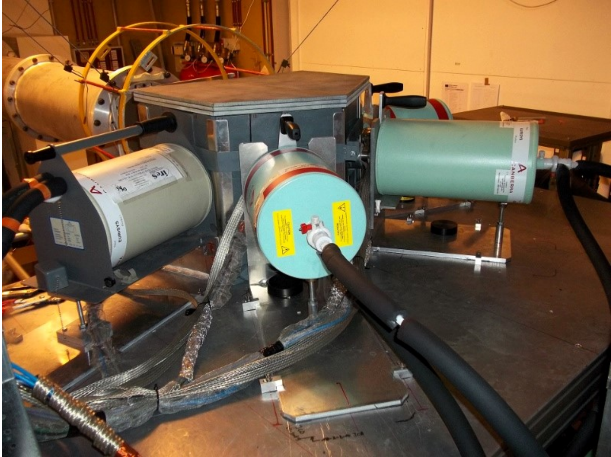
Figure 3: Photography of Grapheme in 2010, at the time when the data analyzed later in this manuscript was recorded. The liquid nitrogen dewars of the HPGe detectors can be seen sticking out of a lead and copper castle shield, with the active Ge crystal being inside, surrounding the target. The neutron beam comes, in the air, from the right and pass through a gap in the shielding (not distinguishable on the picture).
