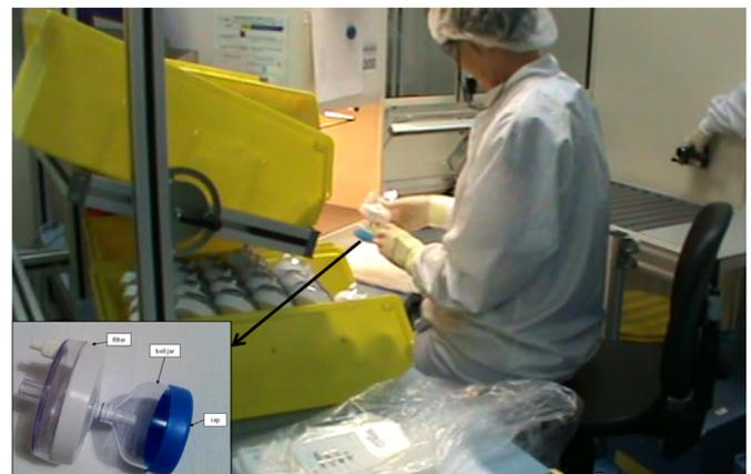
Fig. 1. Workstation dedicated to filter cleaning and description of the filter.
