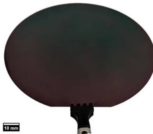
Figure S6-2: Optical image of uniform PGe layer on epi-ready substrate.
