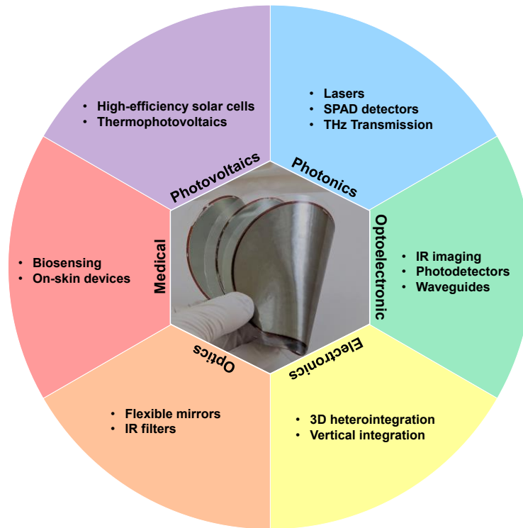
Figure 6-1: Illustration of Ge FSM applications. The central image depicts freestanding Ge membranes on a flexible holder obtained in this work.
