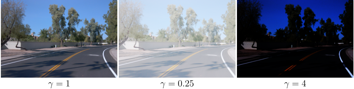
Figure 1.1: Example of a gamma encoding/decoding an image. Source: Waymo dataset [Sun et al. 2020]
