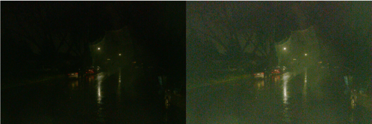
Figure 3: From left to right: example of a night image that we would like to restore and a gamma corrected version of the image showing the high level of noise in the dark regions. Source: Waymo dataset [Sun et al. 2020]
