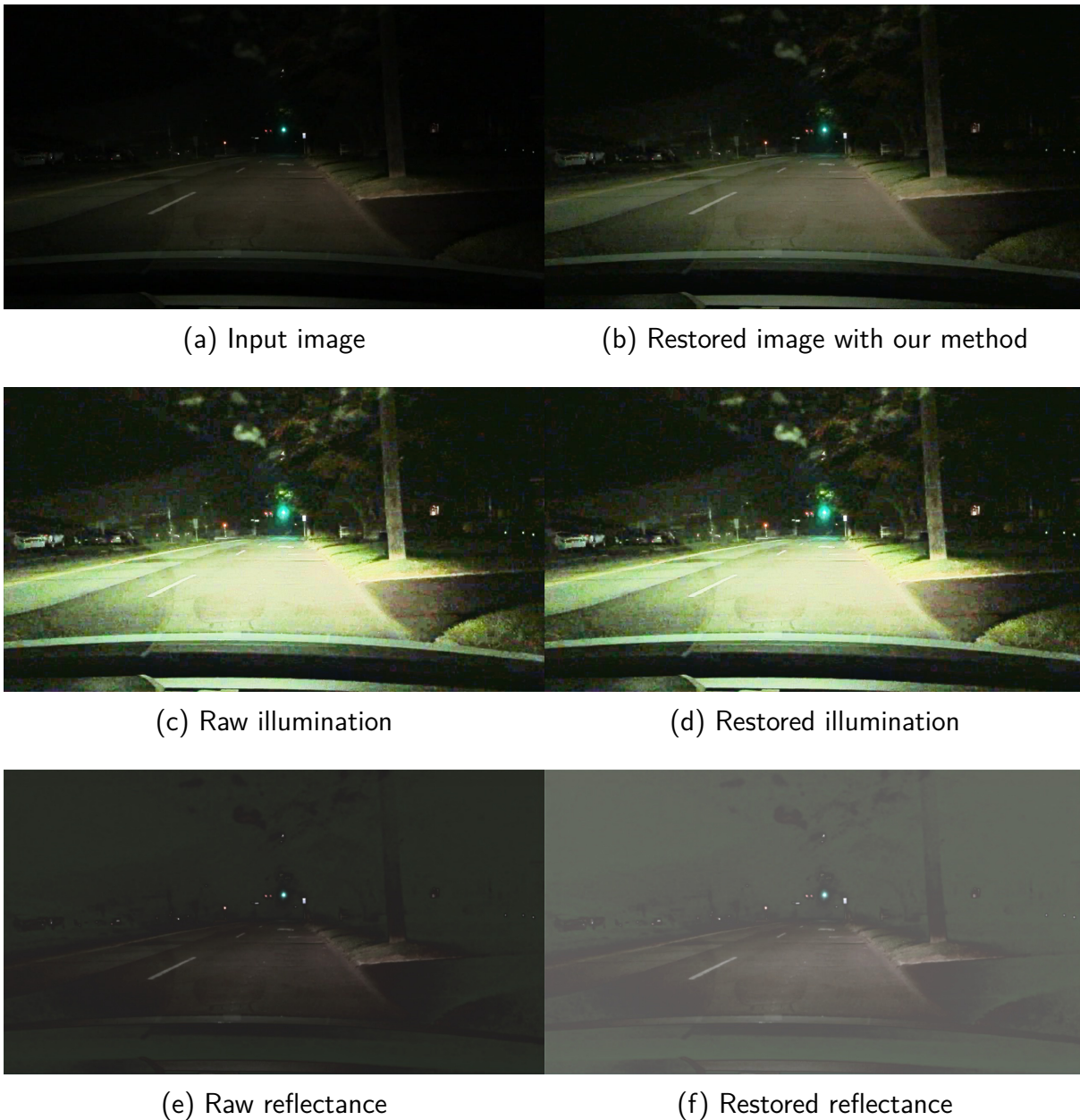
Figure 4.11: An example of the obtained Retinex components and the restoration output on an image coming from the BDD100k dataset [Yu et al. 2020]. We apply the network trained on the Waymo dataset [Sun et al. 2020]. From left column to right column: the input image Fig. 4.11a, the restored image Fig. 4.11b, the extracted raw illumination Fig. 4.11c and its restored version Fig. 4.11d, the extracted raw reflectance and its restored version Figs. 4.11e and 4.11f. The illumination still contains the low-light noise and degradations which strengthen the conclusion on the quality of the decomposition.
