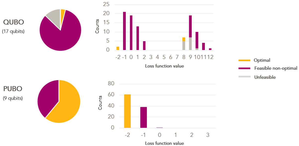
Figure 4.12: Comparison between QUBO and PUBO formulations for Extended Bin Packing on Instance A.
