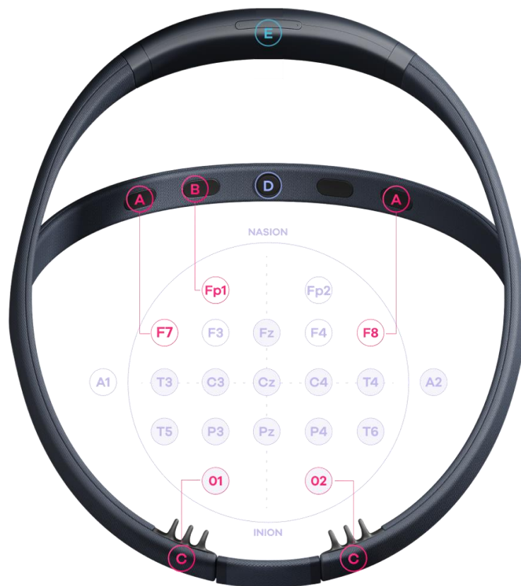
Figure 21. Illustration of the EEG headband and the location of sensors: (A) 2 EEG frontal electrodes, (B) 1 ground EEG electrode, (C) 2 occipital EEG electrodes, (D) bone conduction speaker for audio output, and (E) 3D accelerometer.
