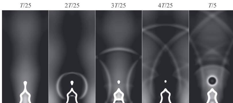
Figure 4.16: Illustration of the numerical experiment. The flame is acoustically forced at St = 0.02 (from [8])
