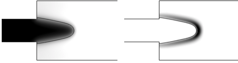
Figure 4.12: Illustration of the 2D axisymmetrical flame used in this study. Left: mean density, Right: mean heat release (from [7])
