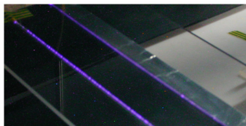
Figure 1.12: Photograph of a wire-to-wire corona discharge: luminous glow is observed in the vicinity of both wires, but brighter near the smaller one (the stressed electrode). Photo taken from [109].
