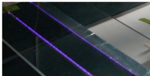
Figure 1.12: Photograph of a wire-to-wire corona discharge: luminous glow is observed in the vicinity of both wires, but brighter near the smaller one (the stressed electrode). Photo taken from [109].
